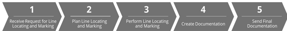
Figure 1: Typical Facility Locating and Marking Process
